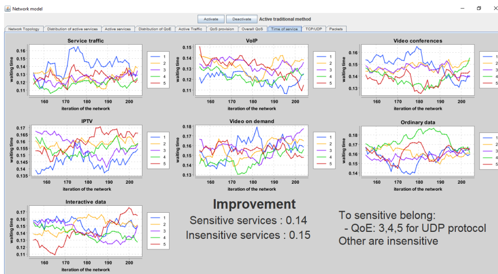
Figure 27. The average waiting time for each session with corresponding QoE score using the traditional method.
